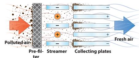
The filter cleaning interval depends on the inlet air pollution density and may vary from 7 up to 21 days. The filter cleaning interval is determined according to the results of the visual inspection of the filters. Vacuum cleaning is allowed.
