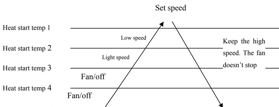
2. 4 minutes after the start up of the indoor fan, the light airflow and the low airflow will be turned to the set speed airflow.
