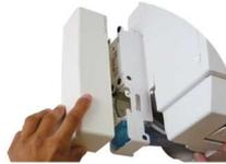
Access to the pump elements (reservoir, tubes etc.) is made by removing the cover.
