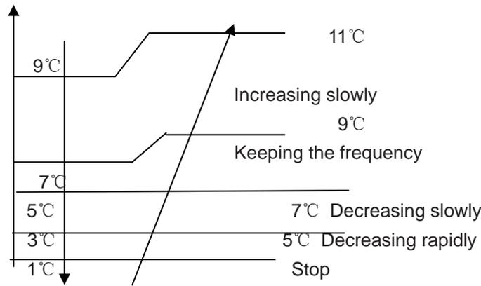
The compressor stops for more than 3 minutes,  $T_{pg\_indoor} > 9^{\circ}\text{C}$ , the compressor recovers.
