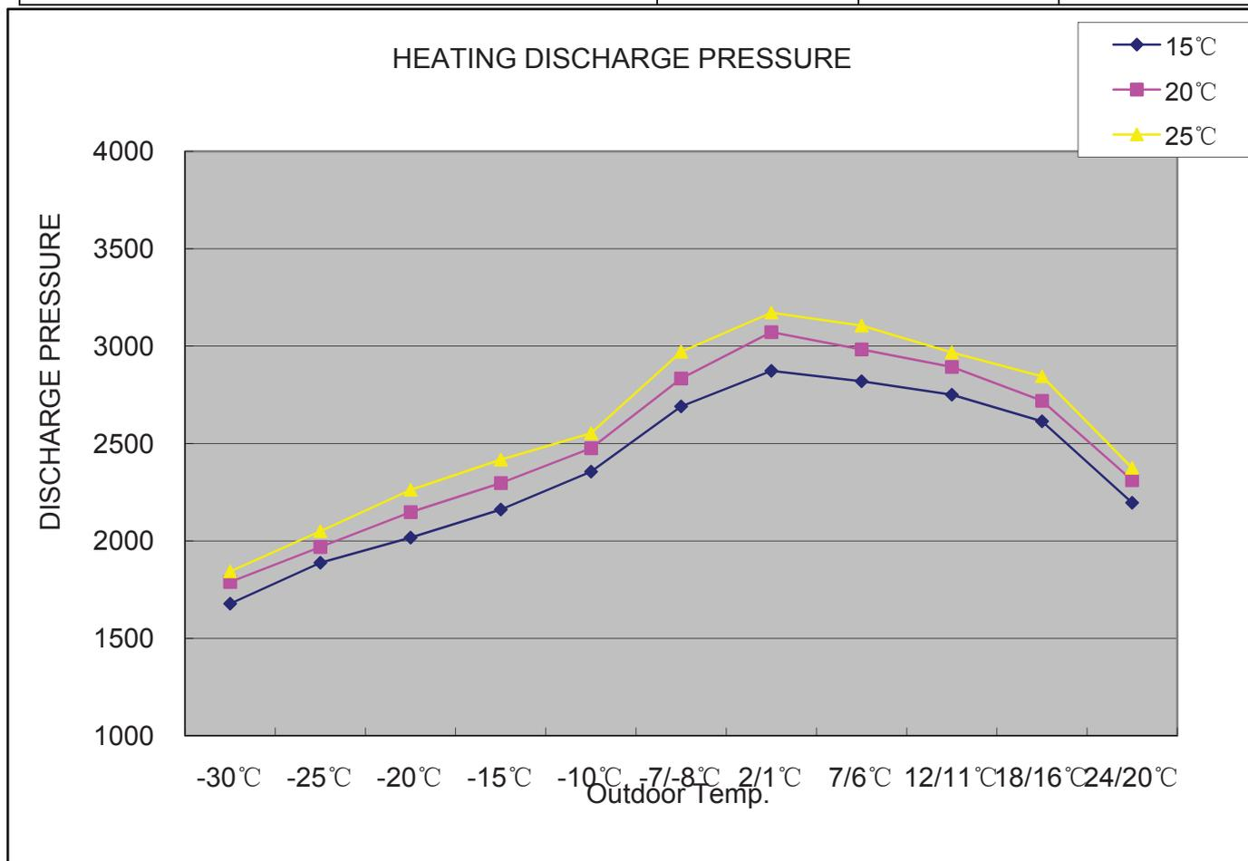
11.7 Heating discharge pressure curves (12K)
