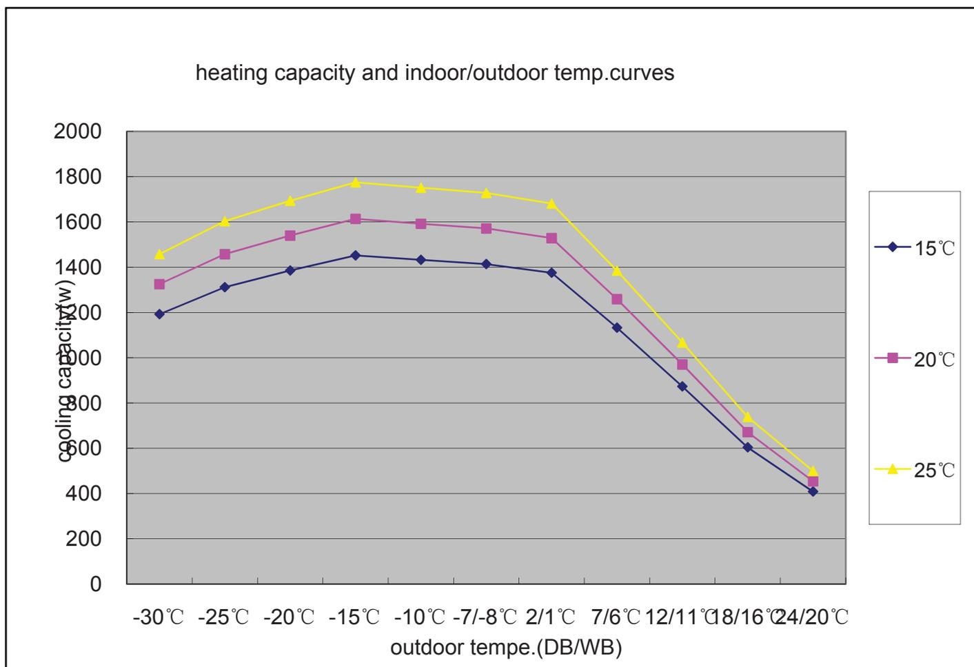
11.6 Heating power consumption value- temperature curves (12K)
