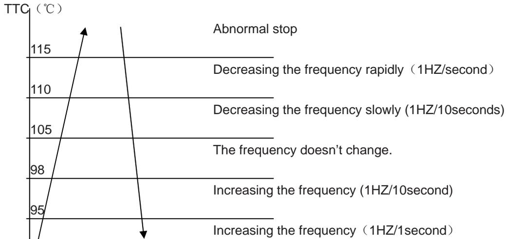
TTC $\geq$ 115 $^{\circ}$ C lasts for 20 seconds. Overheating protection of air-blowing, alarm malfunction to the indoor, others don't last.
