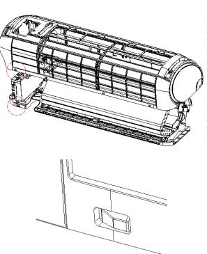
When assembling, install the front grille horizontally so as not to stuff the flap inside.
