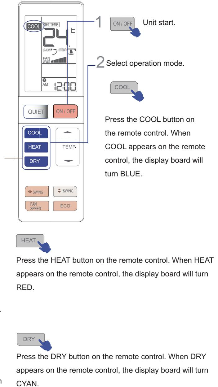
1. In DRY mode, when room temperature becomes lower than temp. setting +2 °C, unit will run intermittently at LOW speed regardless of FAN setting.
