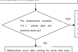
The cryogen may have been leaked during installation, or there may be leakage in the piping system.
